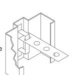
**MASONRY "T"-SHAPED:** A loose metal device used to secure the frame to new masonry walls.
