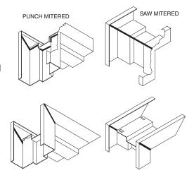
**WELDED**, **FACE**, **FRAME**: Comer/perimeter joints shall have a continuous weld at the faces only.
