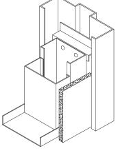
**WOOD STUD:** A metal device secured in a frame to be used for attachment in a wall built with wood studs.
