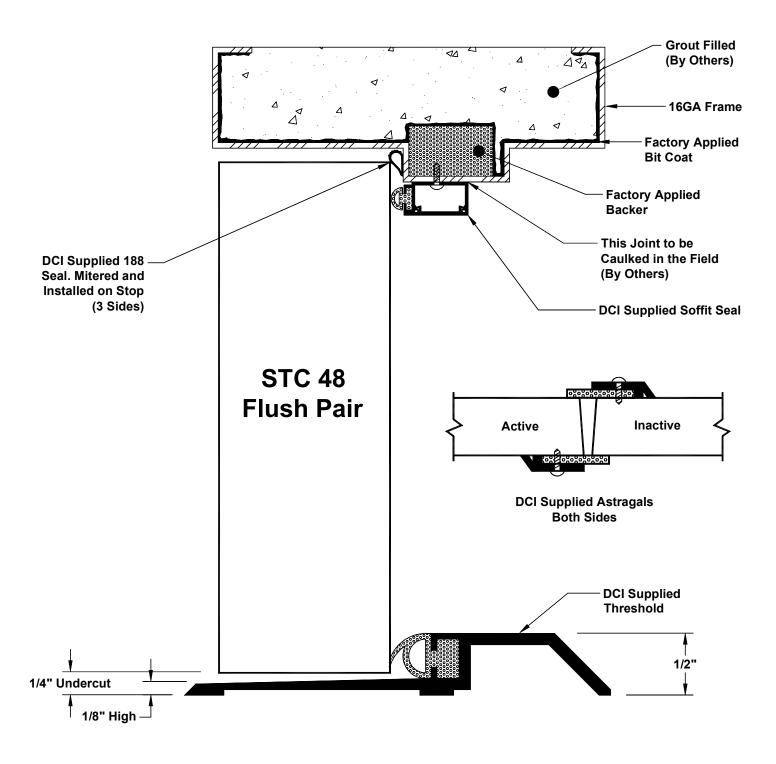
Tested as 6'0"x7'0" with (6) 4-1/2" Hinges, Cylindrical Lock, (2) 6" Manual Flush Bolts
