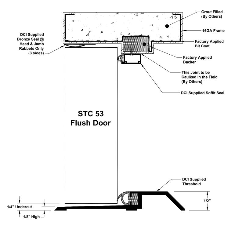
Tested as 3'0"x7'0" with (3) 4-1/2" Hinges, Cylindrical Lock
