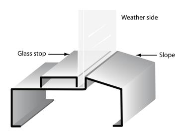
Door Components has designed a unique profile that sheds water and contaminants. This patent-pending design is expected to become the standard in the hollow metal frame industry
