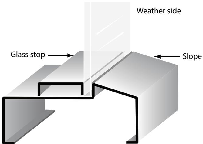
Door Components has designed a unique profile that sheds water and contaminants. This patent-pending design is expected to become the standard in the hollow metal frame industry
